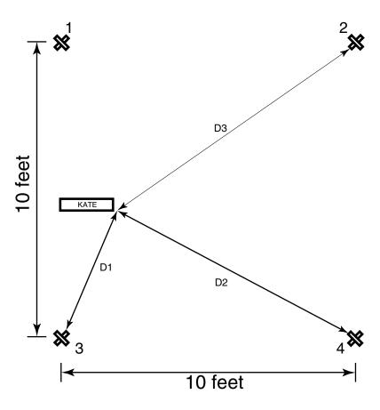
If we draw a reference square using a scale in which one side is equal to 10 feet, then we can use the same scale to draw an arc from corner 3 so that the radius of the arc is equal to D1. Then draw another arc from corner 4 whose radius is equal to D2. The intersection of the two arcs is Kate's estimated position inside the reference square. If we draw a third arc from corner 2 whose radius is equal to D3, the estimated position is more accurate.
